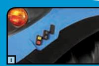
ed on the rear fenders, making it easier to attach implements from the ground (fig. I).
