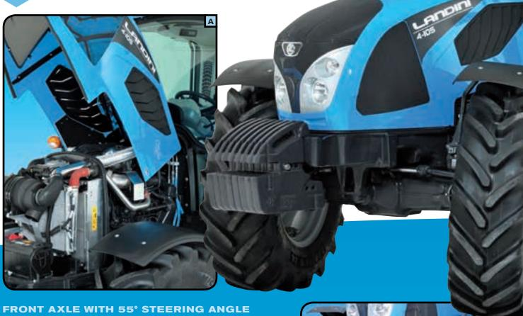
The front axle with electro-hydraulic four-wheel drive engagement offers a 55-degree steering angle providing high ground clearance and excellent manoeuvrability in confined spaces (fig. B). In addition, the combined front and rear wet disc brakes provide efficient and secure all-wheel braking.
